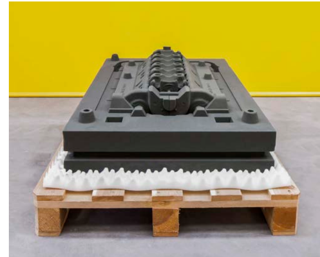
Multi-part sand casting assembly used to cast an engine block. Source: ExOne
